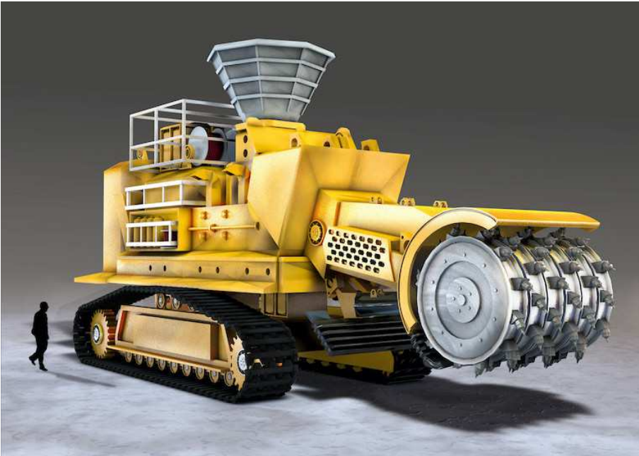
An illustration of a sea mining machine called a bulk cutter, which is intended to pulverize the seafloor for excavation. Image by N.R. Fuller, www.SayoStudio.com .
