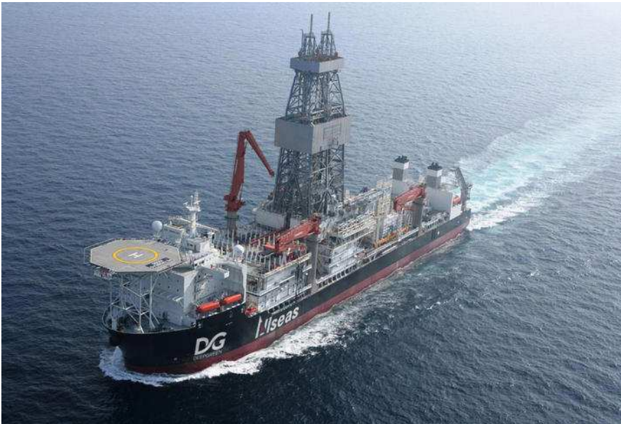
DeepGreen Metals' partner Allseas acquired this former ultra-deepwater drill ship "Vitoria 10000" for conversion to a polymetallic nodule collection vessel. Photo: DeepGreen Metals
