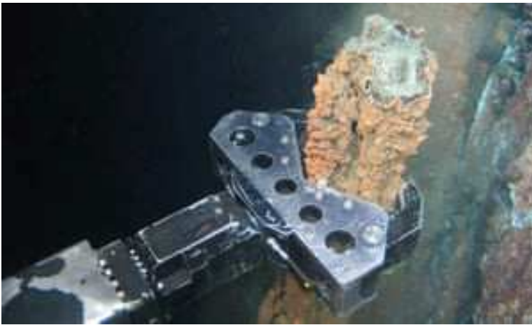
A robotic arm breaks off a chunk of mineral-rich rock for sampling deep underwater off the coast of Papua New Guinea. Photograph: Nautilus Minerals
