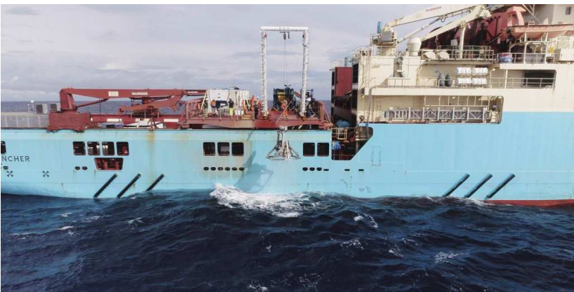
Deployment of box core to collect seafloor polymetallic nodules. DeepGreen
