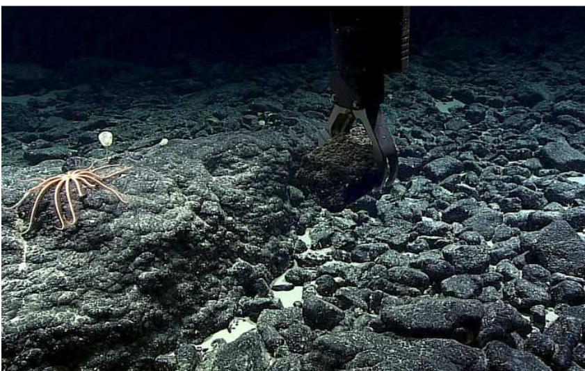
A manganese-crust rock sample being grabbed from the Te Tukunga o Fakahotu dive site, just north of the Manihiki Plateau, near the Cook Islands. Photo: NOAA Office of Ocean Exploration and Research, Mountains in the Deep: Exploring the Central Pacific Basin.
