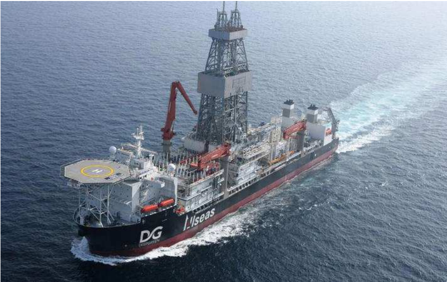
One of the leading advocates of the fledgling deep sea mining sector, DeepGreen Metals hopes to mine the Pacific seabed for polymetallic nodules using collection vessels such as the ultra-deepwater drill ship 'Vitoria 10000'. Photo: DeepGreen Metals
