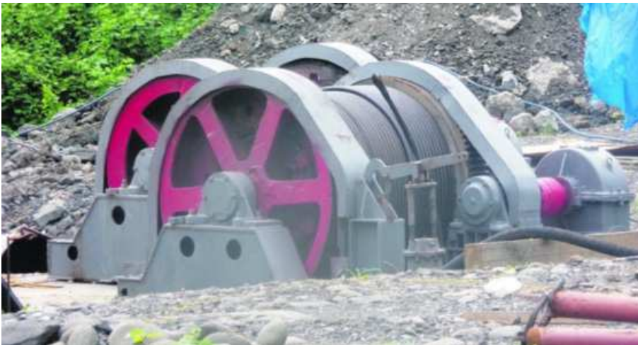
The two cable drums used in the construction of the new Dolphin Shaft. Photo: Charles Chambers
