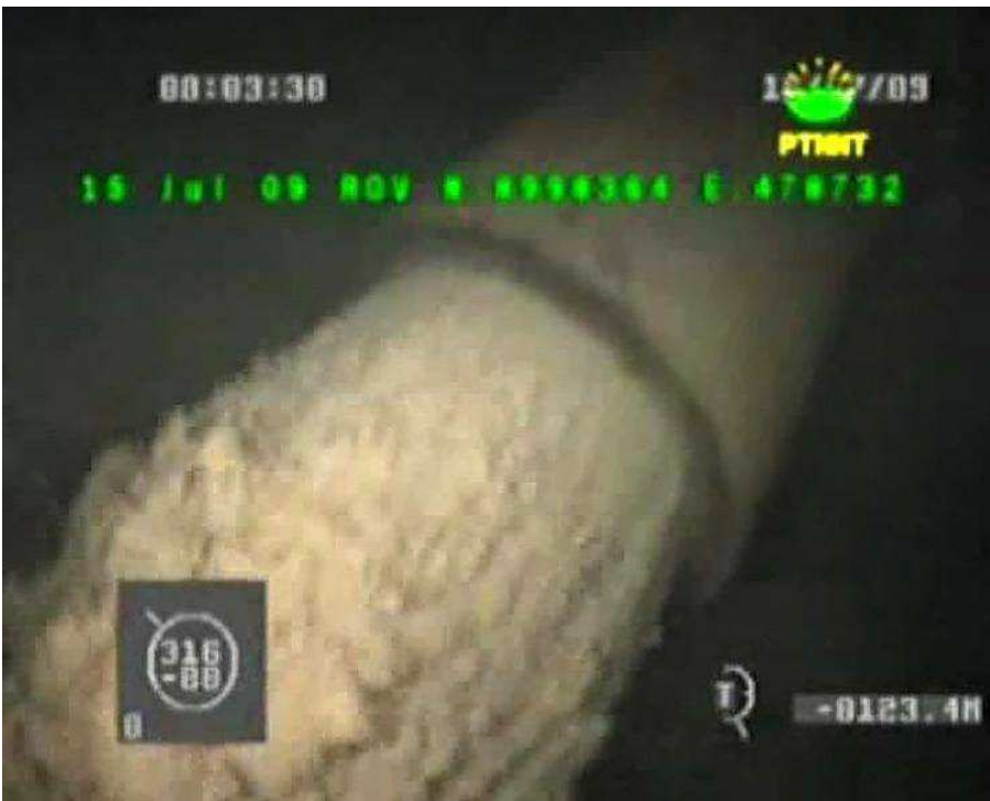
The 4-foot diameter pipe dumping mining wastes into the ocean at Batu Hijau mine in Indonesia.
