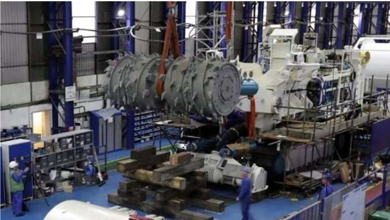
Construction of the largest machine - the 310-tonne Bulk Cutter - was completed in the UK
