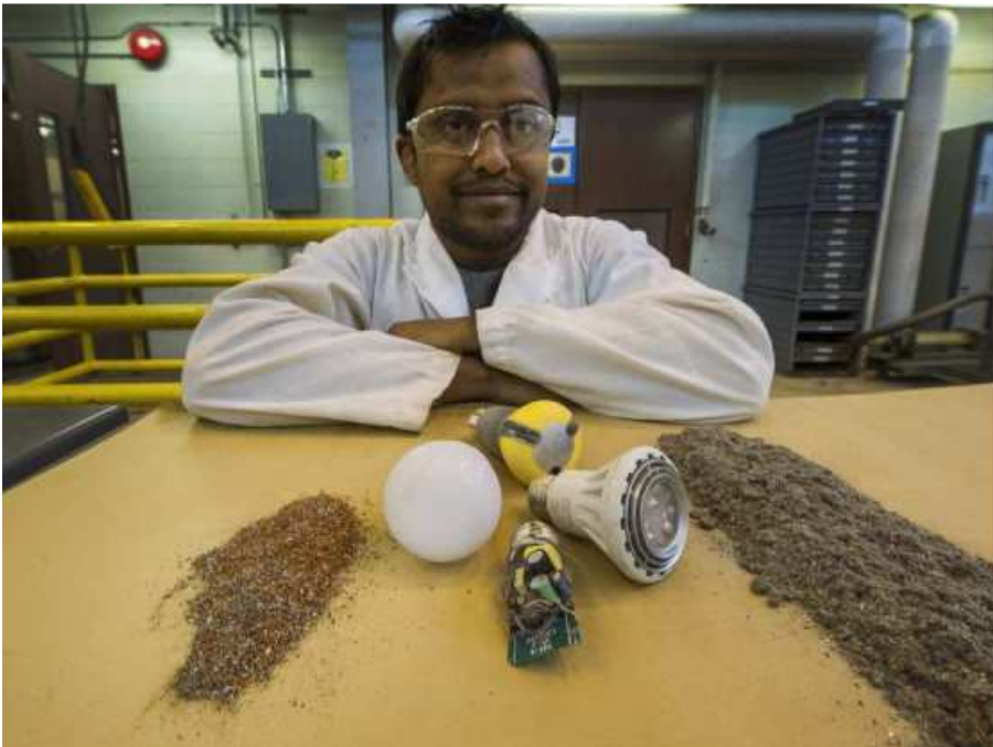
Amit Kumar has been grinding up LEDs at UBC in Vancouver to recover valuable metals. Arlen Redekop
