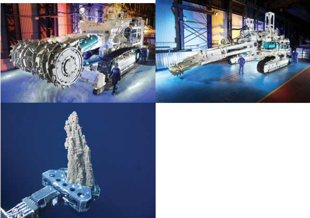
Photos: Nautilus Minerals I, Robot Miner: Three different types of remotely operated machines will be used: a “bulk cutter” [top], a “collecting machine” [center], and an “auxiliary cutter” [see photo “Like A Tank,” above]. Clenched in a manipulator arm is a sample of the kind of metal-rich rock these robots will retrieve from the ocean floor [bottom].
