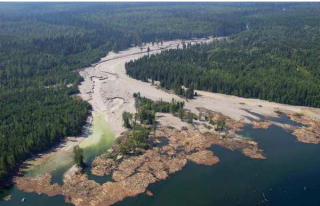
Above: Mine waste and debris enter Quesnel Lake five miles downstream of the failed impoundment at Imperial Metal's Mt. Polley gold/copper mine. Image Credit: Jonathan Hayward, The Canadian Press
